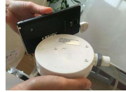
**Note:** Make sure that the NFC reader location is known on the smartphone used. Place the back of the smartphone (where the NFC reader locates) onto the sensor NFC antenna (almost touching) to enable NFC communication.
